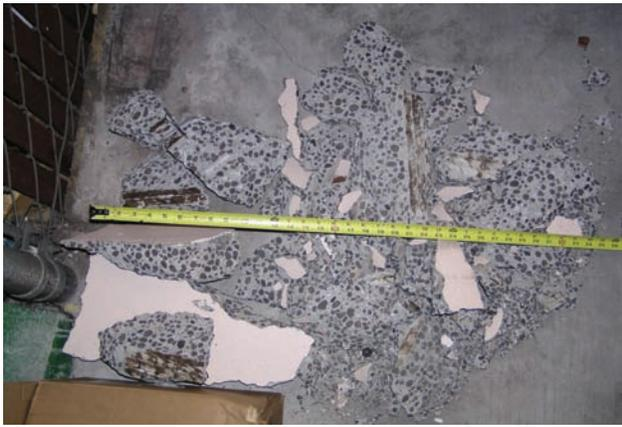
Fig. 1 – Dislodged Concrete
