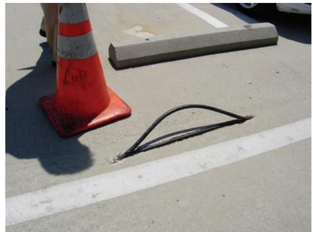
Fig. 4 – A Broken Tendon in Extruded Sheathing
