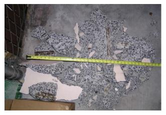
Fig. 1 – Dislodged Concrete
